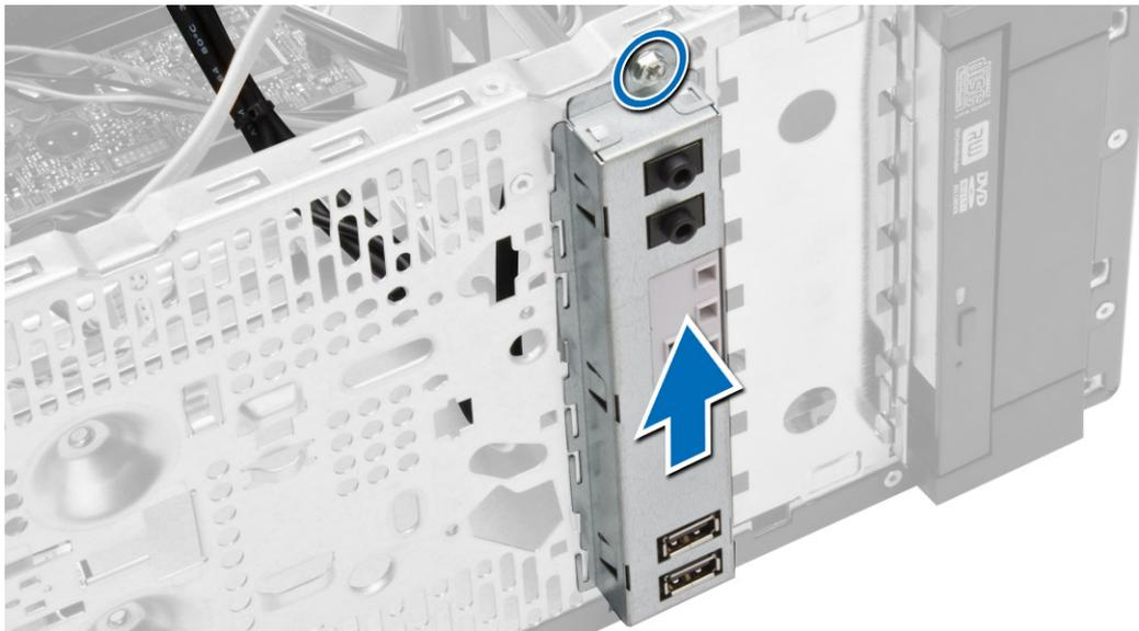
6. Release and pull the I/O panel along with its cable out of the computer.
