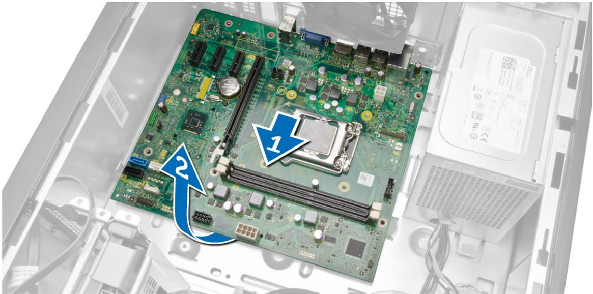
7. Lift the system board out of the computer.
