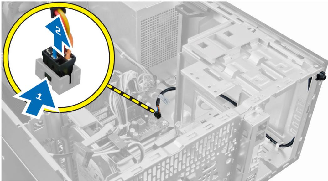
4. Release the power-switch cable from the chassis clips.
