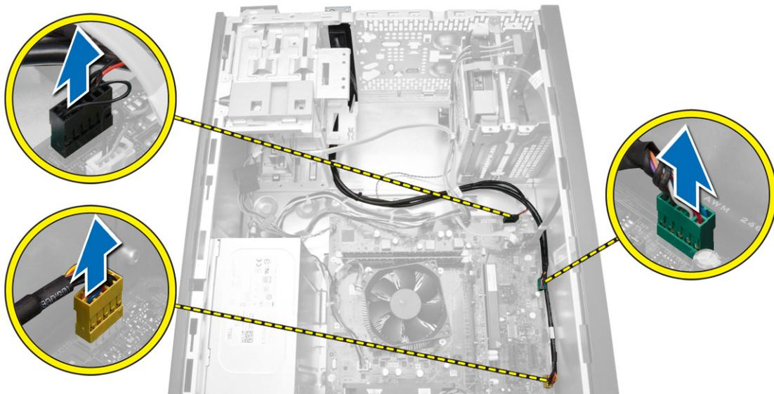
4. Unthread and release the I/O Panel, data cable and USB data cable from the clip on the computer.
